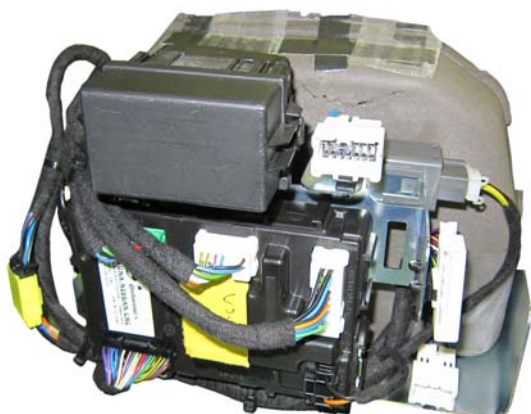
Roof Control Unit
