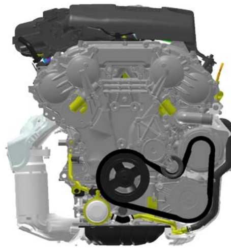
Pathfinder Belt Routing (no power steering pulley)
