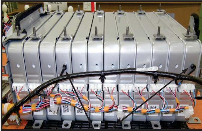
Battery Pack Temperature Sensors
