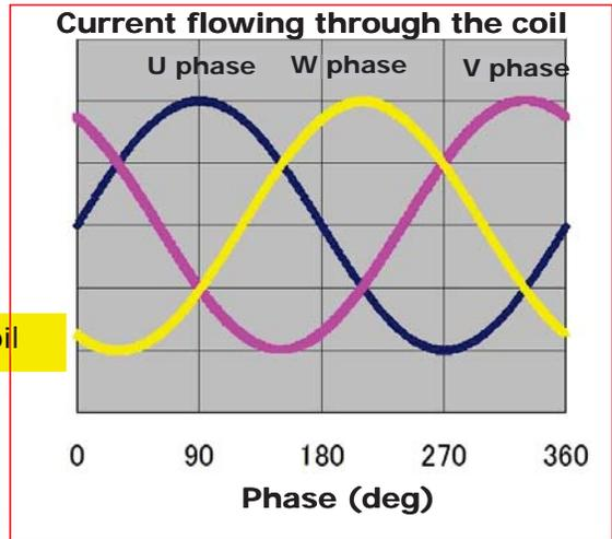
**Rotation of Permanent Magnet Synchronous Motor**
