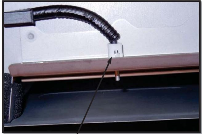
Battery Cooling Intake Temp Sensor (Q50 only)
