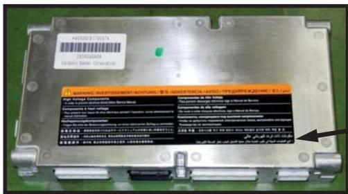
Lithium-ion Battery Controller (LBC) Warning Label
