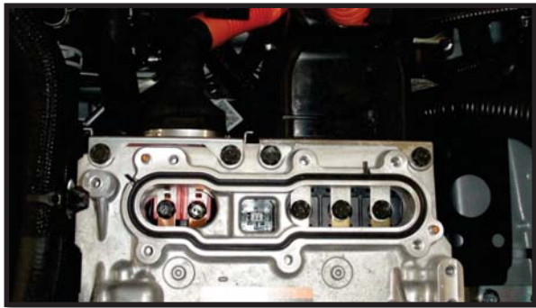
High-voltage Cover Removed
